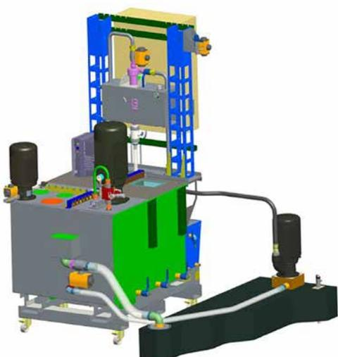
The image shows a complete IFDR 500/32 solution fitted with a delivery pump 20 bar 35 L/min and a delivery pump 70 bar managed by the inverter and the proportional valve, programmed to perform 6 pressure steps at these values: 20, 30, 40, 50, 60, 70 bar with maximum flow rate 52 L/min.
