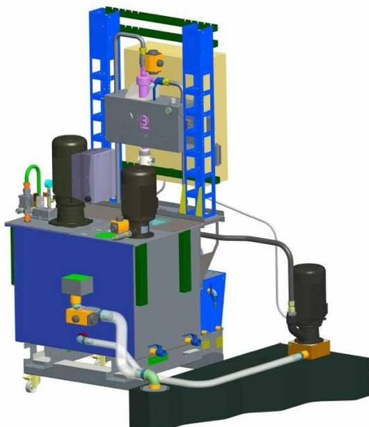
The image shows a complete IFDR 300/20 fine filtration system fitted with a delivery pump 20 bar 35 L/min and a delivery pump 70 bar managed by the inverter and the proportional valve, programmed to perform 6 pressure steps at these values: 20, 30, 40, 50, 60, 70 bar with maximum flow rate 33 L/min.
